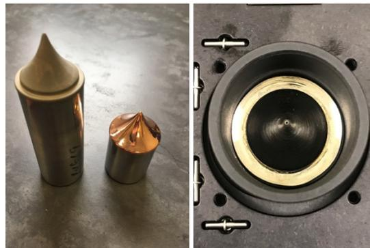
Figure 1: Butler baffles on mandrels (L) and after polishing, blackening, and mounting for optical testing (R).
