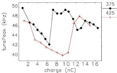
Figure 4: Measured synchrotron tune peak frequency vs. charge at two beam energies.
