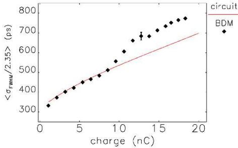
Figure 3: Bunch length comparisons of measurements and circuit model for 425 MeV, using natural energy spread.
