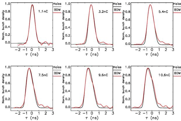
Figure 2: Haissinski fits to measured beam distributions.
