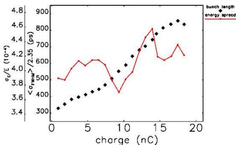
Figure 7: Bunch length and energy spread measured at the same time, 425 MeV.
