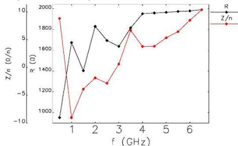
Figure 9: Running average of the real part, and running slope of the imaginary part divided by  $n$ , of the PAR numerical impedance in [8]. Frequency steps are 500 MHz.
