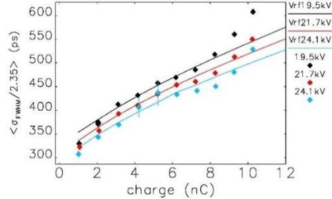
Figure 5: Variation of bunch length with harmonic rf voltage after compression; comparison of circuit model (lines) with measurements (symbols).
