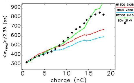
Figure 8: Bunch length comparisons of measured BDM data and circuit models for 425 MeV, using measured energy spread.
