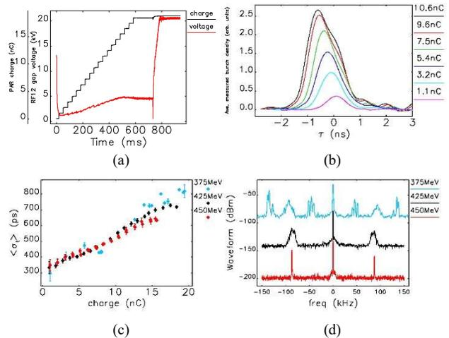
Figure 1: PAR measurements: (a) charge and harmonic rf waveform over cycle, (b) bunch distributions, (c) rms bunch length, and (d) synchrotron tune spectra for 16nC.
