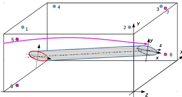
Figure 3: Schematic diagram of septum magnet geometry and eight fiducial markers. Only the stored beam chamber is illustrated. The injected beam chamber will be a similar box as the magnet itself.
