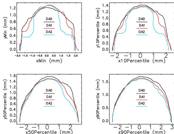
Figure 6: Simulated DA: DA0 - without septum leakage field; DA1 - with calculated septum leakage field; DA2 - Septum leakage field error doubled.
