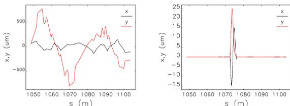
Figure 5: Closed orbit without (left) and with (right) septum leakage field correction.
