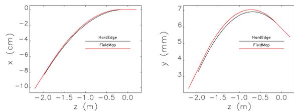
Figure 4: Calculated injected beam orbit from hard edge model (black), and designed septum magnetic field map (red).
