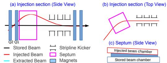
Figure 1: Schematic drawing of injection region and septum placement. (a) The septum has a roll angle to provide a gentle vertical bend; (b) The septum has a yaw angle; (c) The septum has a pitch angle to reduce the leakage field.
