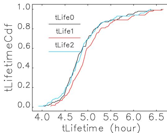
Figure 7: Simulated cumulative Touschek lifetime distribution: tLife0 - without septum leakage field; tLife1 - with calculated septum leakage field; tLife2 - Septum leakage field error doubled.
