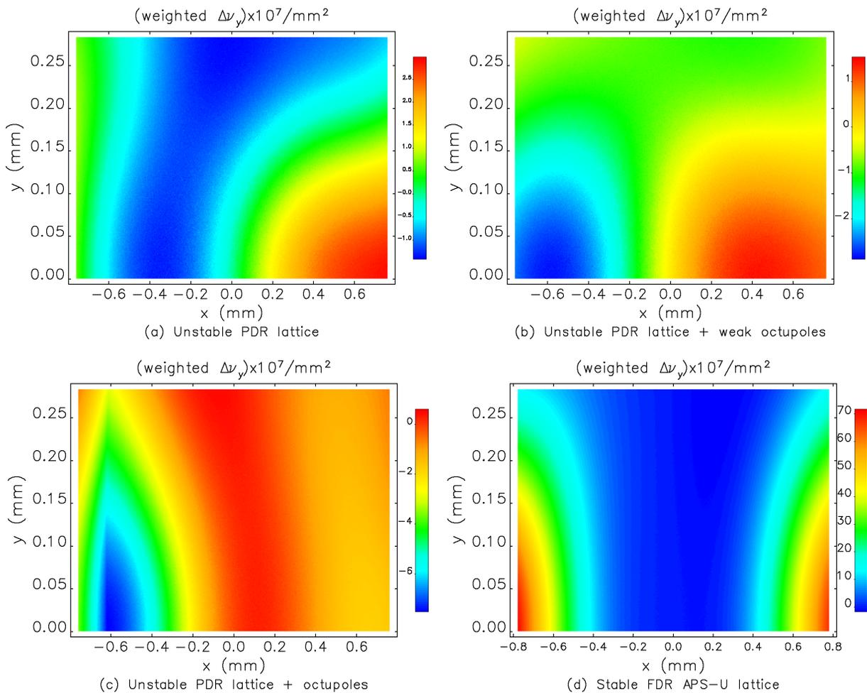
Figure 2: Vertical tune shift weighted by the local particle density in  $1/\text{mm}^2$ . The spread in weighted  $\Delta\nu_y$  for the two unstable cases in (a) and (b) are comparable, and noticeably smaller than that of the PDR lattice with stabilizing octupoles in panel (c). The stable FDR lattice has a significantly larger tune shift as shown in (d).
