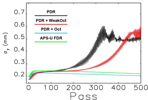
Figure 1: Vertical beam size after injection for the PDR lattice (black), the PDR lattice including weak octupoles (red), the PDR with stronger octupoles (blue), and the FDR lattice (green). The first two cases suffer significant particle loss, while the other two are stable.
