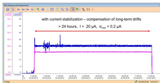
Figure 5: Beam current measured from cathode and collected by the Faraday cup. The beam loss from cathode to FC is 5%. The rest difference in between is due to some calibration issue. A high stability of 1% is kept in 24 hours of continuous operation.
