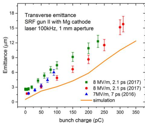
Figure 3: Measured transverse emittance vs. bunch charge, compared with the ASTRA simulation result.
