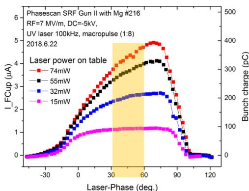
Figure 2: Measured Faraday cup current (and bunch charge) vs. drive laser phase. The working laser phase of the SRF gun is indicated by the vertical zone (40° to 60°).
