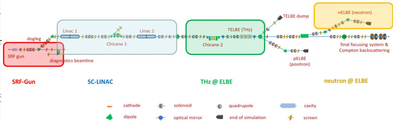
Figure 6: Layout of the SRF gun and SRF linac followed by THz beam line (TELBE) and neutron beam line (nELBE).
