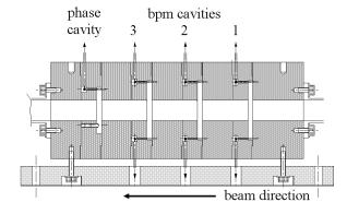
Figure 1. Mechanical drawing of the triplet RF-BPM set used for measuring the BPMs' resolutions.
