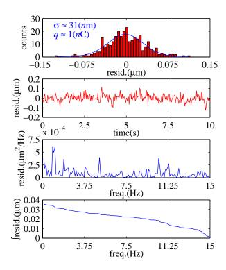
Figure 3. The histogram, time and frequency structure, and integrated amplitude of the residual from top to bottom, respectively.
