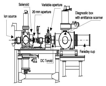
Figure 1. CDS injector and diagnostic station.
