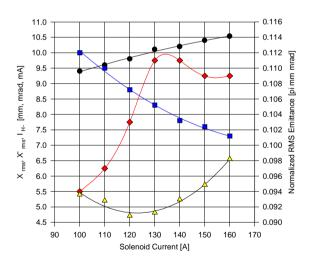
Figure 4. Beam parameters vs. Solenoid current. ( $\bullet$ ) Ion current; ( $\blacksquare$ ) rms beam size; ( $\blacktriangle$ ) rms divergence; ( $\blacklozenge$ ) normalized rms emittance. Variable aperture = 40 x 40 mm<sup>2</sup>.
