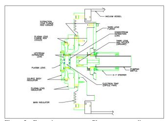
Figure 2. Extraction geometry. Plasma aperture diameter = 13 mm, first accelerating gap = 5.5 mm, extraction lens upstream aperture diameter = 9.5 mm, second accelerating gap = 19.35 mm, extraction lens upstream aperture diameter = ground electrode aperture diameter = 14.0 mm
