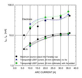
Figure 3. Ion and electron current vs. Arc current. ( $\bullet$ ) Extraction directly into faraday cup. Transported LEBT current with: ( $\blacktriangle$ ) residual H2; ( $\blacklozenge$ ) Xe gas added to LEBT. Solenoid current = 160 A. Beam energy = 40 kV.
