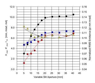
Figure 5. Beam parameters vs. Variable aperture opening. ( $\bigcirc$ ) Ion current; ( $\blacksquare$ ) rms beam size; ( $\blacktriangle$ ) rms divergence; ( $\diamondsuit$ ) normalized rms emittance. Solenoid current = 160 A.
