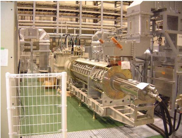
Figure 5: The klystron under high-power test
