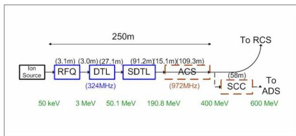
Figure 3: Scheme of J-PARC Linac
