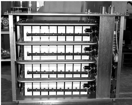
Figure 4: Pulse Forming Network / Marx
