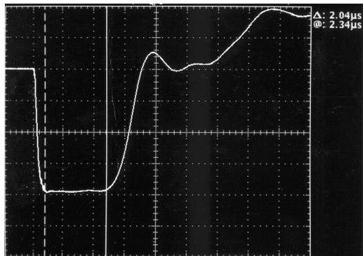
Figure 5: Full Voltage Pulse with Initial Compensation Resistance
