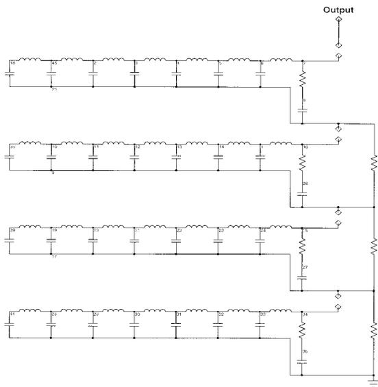
Figure 3: PFN / Marx Schematic
