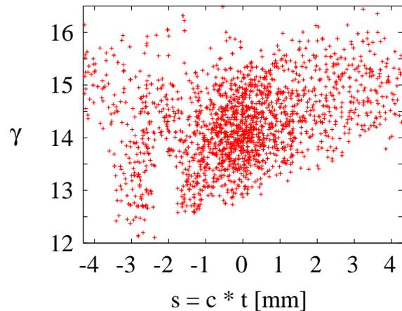
Figure 5: Longitudinal phase space distribution at wiggler exit.
