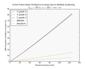
Figure 1: Beam emittance increases as a function of vacuum window thickness (in thousandths of an inch) for different common materials.
