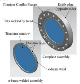
Figure 2: Titanium vacuum window assembly.
