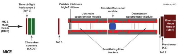
Figure 1: The MICE Beamline. Experimental data was gathered with various absorbers such as liquid Hydrogen, Lithium Hydride and a Polyethylene wedge. The beam was tracked through the spectrometer solenoids at each of the five upstream and downstream scintillating fibre stations.
