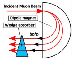
Figure 3: Emittance Exchange between the longitudinal and transverse phase-space.
