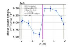
Figure 7: Change in the transverse phase-space density from the upstream reference plane to the downstream reference plane.
