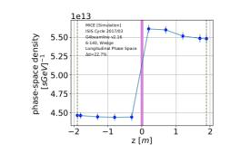
Figure 6: MICE simulation. Increase in the longitudinal phase-space density from the upstream reference plane to the downstream reference plane after passing through the wedge.
