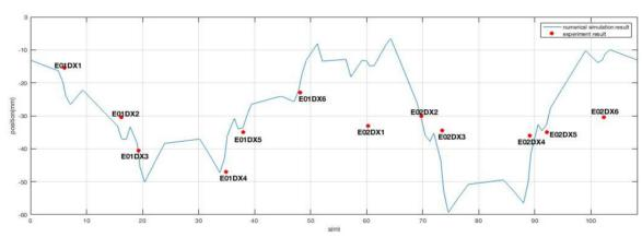
Figure 3: Numerical simulation in ELEGANT and experimental result are shown. The red points are the experimental results and the blue solid line is the ELEGANT simulation. Experiment and simulation are done for an off-momentum particle (dp/p=1%).
