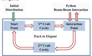
Figure 2: Simulation flow for beam-beam interaction.
