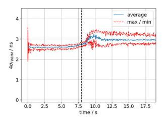
Figure 1: Measured  $4\sigma_{\text{FWHM}}$  bunch length of 12 bunches at flat bottom. The vertical dashed line indicates the time at which the threshold condition in Eq. (1) is satisfied.
