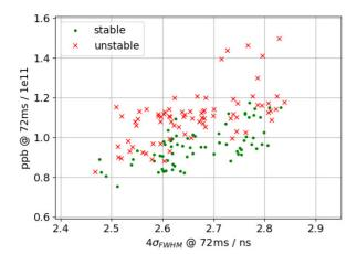
Figure 2: Measured instability thresholds as a function of bunch length for 12 bunches without feedback. With feedback on, beams were stable up to  $2.2 \times 10^{11}$  ppb.
