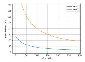
Figure 6: Coupled bunch instability growth time versus TWC detuning  $\Delta f_r$  for multipoles m = 1, 2.
