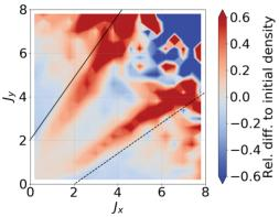
Figure 4: Relative change of the bunch distribution from an initially Gaussian bunch, in normalised transverse action  $\stackrel{\mathbf{Z}}{=}$  space  $(J_x, J_y)$ , in a simulation including external noise and impedance. The black solid (dashed) line shows the actions that correspond to the most unstable mode in the horizontal (vertical) plane. Courtesy of X. Buffat [6].
