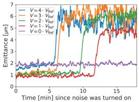
Figure 1: Evolution of normalised horizontal emittance for 5 bunches in beam 2, with linearly spaced external noise amplitudes.  $I_{\rm oct} = 452 \, \text{A}$ ,  $Q' \approx 15$ , and  $\tau_g \sim 200 \, \text{turns}$ .
