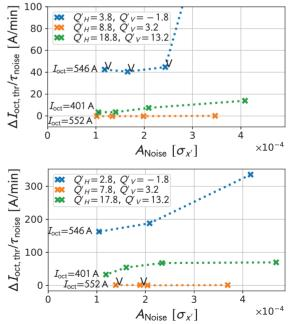
Figure 3: Scan of chromaticity in both beams. Beam 1 is on top, where the last point is at  $(4.7 \times 10^{-4} \, \sigma_{X'}, 404 \, \text{A/min})$ . Beam 2 is below. The points marked with a 'V' became unstable vertically. The values for  $I_{\text{oct}}$  when the noise was turned on are annotated next to the lines. The damping time was  $\tau_g \sim 200 \, \text{turns}$ .
