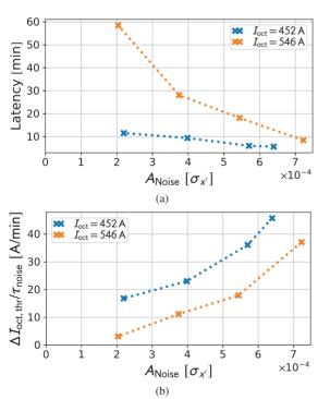
Figure 2: Scan of octupole current in beam 2, with a chromaticity  $Q' \approx 15$  and damping time  $\tau_g \sim 200$  turns in both transverse planes. The values for  $I_{\rm oct}$  when the noise was turned on is given in the legends. (a) shows the latency. (b) shows the rate of change of the stability threshold.
