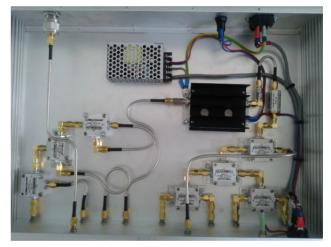
Figure 2: Inside of the MO divider.
