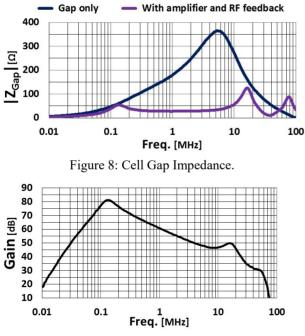
Figure 9: Cell Transfer Function.
