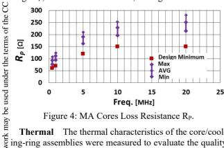
Figure 4: MA Cores Loss Resistance R<sub>P</sub>.
