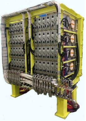
Figure 2: Cavities grouping for one PSB Straight Section.
