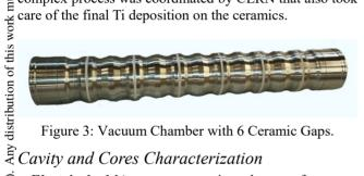
Figure 3: Vacuum Chamber with 6 Ceramic Gaps.
