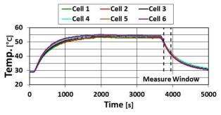
Figure 6: Thermal Transient for the Evaluation of the Water Sharing among Cells in one Cavity.
