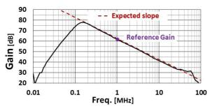
Figure 7: Power Amplifier Frequency Response.
