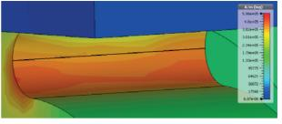
Figure 8: Tangential magnetic field at slot edge.
