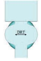
Figure 4: coupler geometry. DRT parameter is indicated.
