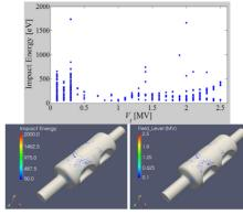
Figure 4: Impact energy vs. voltage and resonant particle locations.
