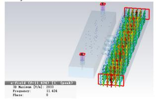
Figure 5: Electric field of H-plane directional coupler by
