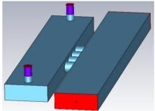
Figure 1: H-plane directional coupler in CST.
