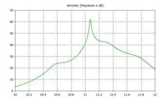
Figure 11: Directivity of circular-rectangle waveguide directional coupler by CST.
