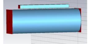
Figure 8: Circular-rectangle waveguide directional coupler in CST.
