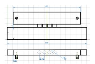
Figure 4: Main dimensions of H-plane directional coupler (units: mm).
