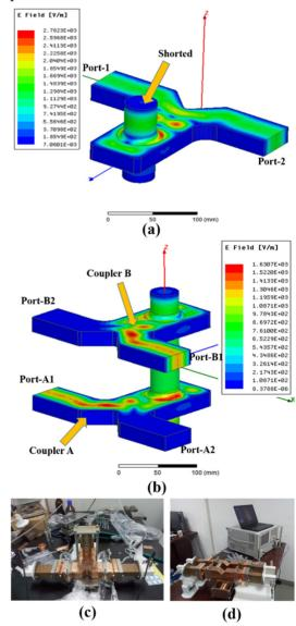
Figure 1: Two methods of measuring the coupler: (a) shortcircuiting the circular waveguide and (b) connecting two couplers to form one through the circular waveguide. (c) and (d) are the corresponding physical setup.
