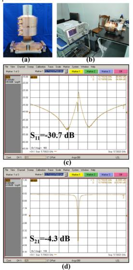
Figure 2: (a) Spherical pulse compressor prototype, (b) RF measurement of the prototype, (c) the reflection is -30.7 dB and (d) the transmission is -4.3 dB after tuning.
