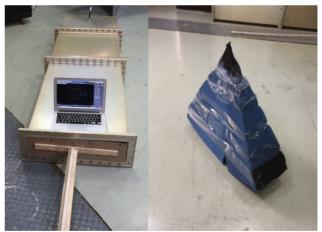
Figure 2: The self-reflection measurement configuration of the coaxial-waveguide converter (left); a kind of split-type carbon powder absorbing load (right).
