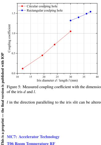
Figure 5: Measured coupling coefficient with the dimension of the iris d and l.
