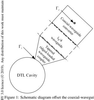
Figure 1: Schematic diagram offset the coaxial-waveguide 20 convert reflection with  $\lambda_g/4$ .
