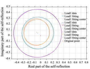
Figure 3: Measurement result of the self-reflection of the coaxial-waveguide converter with three different shape of the split-type carbon powder loads.
