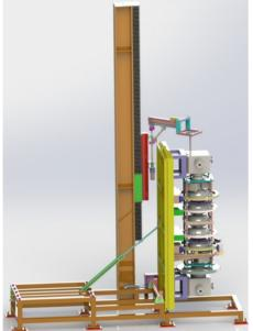
Figure 1: Mechanical rotation and turning platform.
