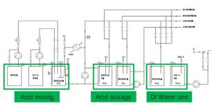
Figure 2: Schematic diagram of electrolyte preparation and equipment cleaning unit.
