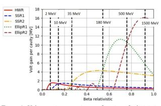
Figure 1: Voltage gain per cavity as a function of relativistic beta for the JAEA-ADS project.
