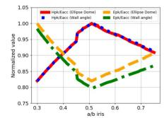
work Figure 3: The electromagnetic peaks as a function of the iris ratio by adjusting the ellipse dome ratio (solid red line and this dashed orange line) and adjusting  $\alpha$  (dotted blue line and dashed-dotted green line) to tune the frequency . The valt from ues were normalized to maximum value of electromagnetic peaks.
