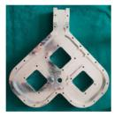
(b) Slotted plane of the Mode Launcher.
