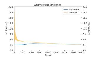
Figure 8: Vertical and horizontal emittance versus turn number after injection at 6 GeV for the bare Q40 optics,  $Q'_{x,y} = -5$  with transverse damper, at  $N_b = 2 \times 10^{10}$ .
