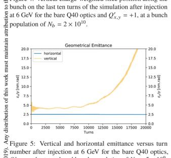
Figure 5: Vertical and horizontal emittance versus turn in number after injection at 6 GeV for the bare Q40 optics,  $Q'_{x,y} = +1$ , at a reduced bunch population of  $N_b = 5 \times 10^9$ . CONCLUSIONS Our simulations suggest that operating the bare SPS Q40 Contice as PBR for leptons with a fast turn-by-turn damper at
