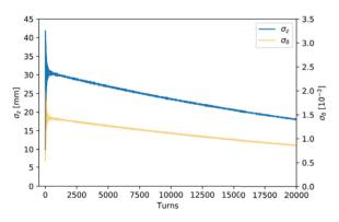
Figure 1: Electron rms bunch length and energy spread vs. turn number after 6 GeV injection for the bare Q40 optics.
