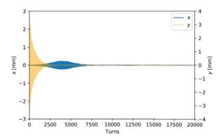
Figure 7: Vertical and horizontal bunch centroid position versus turn number after injection at 6 GeV for the bare Q40 optics,  $Q'_{x,y} = -5$  with transverse damper, at  $N_b = 2 \times 10^{10}$ .
