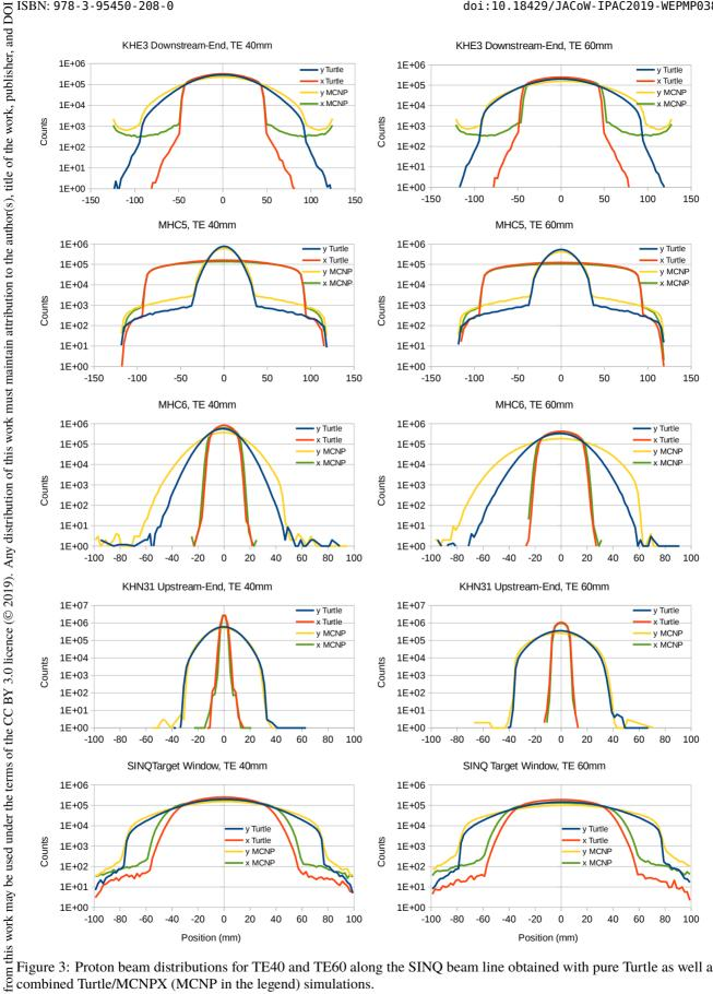
Figure 3: Proton beam distributions for TE40 and TE60 along the SINQ beam line obtained with pure Turtle as well as combined Turtle/MCNPX (MCNP in the legend) simulations.
