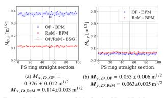
Figure 3: Measurements of  $M_D$  for the OP and ReM optics in the (a) horizontal and (b) vertical planes.
