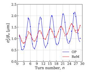
Figure 4: Turn-by-turn beam profile measurements after injection.
