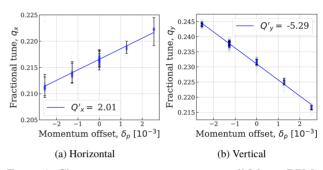
Figure 1: Chromaticity measurement using all 86 ring BPMs during the first 30 turns.
