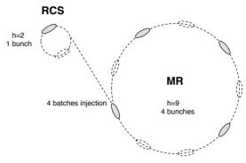
Figure 1: Beam transfer diagram from RCS to MR for COMET.
