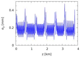
Figure 3: RHIC's most probable vertical orbit excursion around the ring with an rms value of 200 µm.
