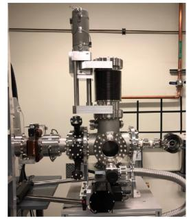
Figure 4: Assembled BID chamber. Visible from left to right: in-flange ACCT, bellows with X-Y steerer, 4-way X-Y BPM, blackened through ports on imaging octagon, 6way cross housing full power beam dump and turbomolecular pumping, temporary beam dump with ceramic standoffs for Faraday cup measurement of current including a cooling fan.
