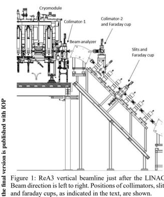
Figure 1: ReA3 vertical beamline just after the LINAC. Beam direction is left to right. Positions of collimators, slits and faraday cups, as indicated in the text, are shown.
