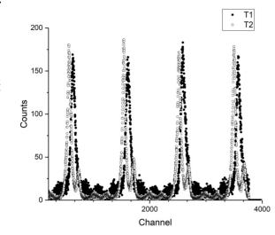
Figure 3: BaF2 timing spectrum with peaks related to times T1 (closed dots) and T2 (open dots) of equation (1). Note  $\frac{1}{2}$  T1 (closed dots) and T2 (open dots) of equation (1). Note that the second smaller peak in T2 is spurious, correspond- $\frac{1}{2}$  ing to a small amount of the beam hitting an obstacle in the beam line prior to the beam stopper.
