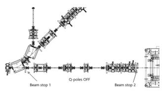
Figure 2: Horizontal beam line where time-of-flight measurement was performed. Beam direction is left to right.
