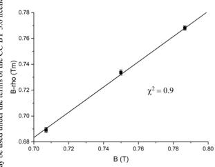
B (T) Figure 4: Magnetic rigidity (B-rho) deduced from time-of-flight measurements as a function of the measured field in the magnet (B). The line corresponds to the best fit.
