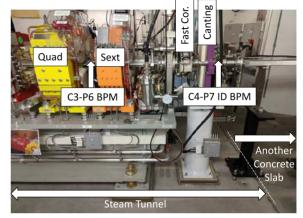
Figure 9: Relative positions of one ID BPM (C4-P7), one bounding BPM (C3-P6), different types of magnets, and the steam tunnel (extending beyond the left edge and separated by 635-mm-thick accelerator tunnel concreate floor). C04 ID is located on the right side of photo.
