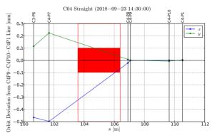
Figure 10: Estimated physical BPM motions for C3-P6 and C4-P7 assuming C4-P9, C4-P10 and C4-P1 were stable (C04 ID represented by red box).
