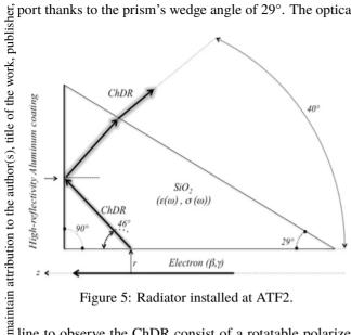
Figure 5: Radiator installed at ATF2.
