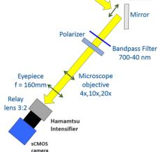
Figure 7: New optical line at ATF2. The yellow arrows represent the ChDR light path.
