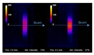
Figure 2: ChDR light recorded on the camera for a beam to dielectric distance of 3 mm (left) and 0.5 mm (right).
