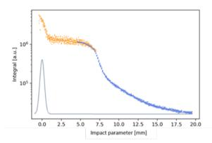
Figure 3: Impact parameter scan against total intensity of ChDR. The approximate beam profile is shown in grey.
