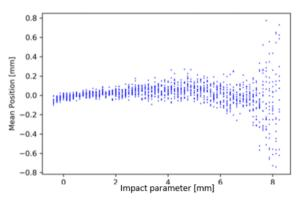
Figure 4: Vertical position of the beam during the impact parameter scan.
