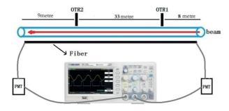
Figure 3: Scheme of the CBLM installed at BEPC II linac.
