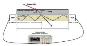
Figure 1: Scheme of beam loss monitor.
