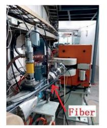
Figure 2: Black cables mounted on the side of the vacuum chamber are the optical fibers for the loss monitor.
