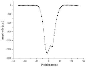
Figure 6: Positive ions distribution at MEBT.
