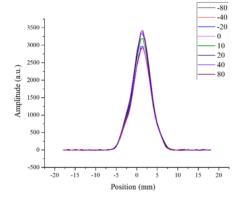
Figure 8: Horizontal profile measurement results under different bias voltage at CSNS-LRBT.
