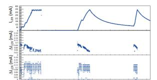
Figure 2: Time chart of operation current and injected currents at LER: The top plot shows the operation current. The middle and bottom plots are the injected currents determined with ordinary and new methods, respectively. The data from June 1st 22:00 to June 2nd 2:00 in 2018 are shown.
