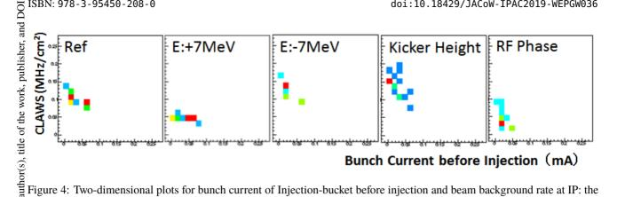
Figure 4: Two-dimensional plots for bunch current of Injection-bucket before injection and beam background rate at IP: the data in the injection conditions of normal parameters, injection bunch energy +7 MeV and -7 MeV, injection kicker height -0.75 mm, and RF phase at HER +4 degrees are shown. The number of entries in each bin is illustrated with colors. The red indicates large entries while the blue indicates a few entries.
