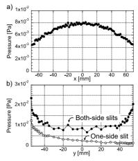
Figure 3: Calculated pressure distribution along a) the x-axis and b) the y-axis.
