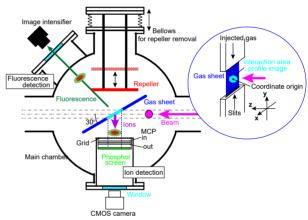
Figure 1: Conceptional diagram of a gas-sheet based beam profile monitor in J-PARC LINAC.
