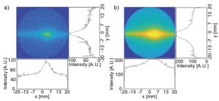
Figure 5: Typical beam profile for the different applied voltages on the MCP input. a)  $V_{\text{MCP}_{in}}$ =-1150 V. b)  $V_{\text{MCP}_{in}}$ =-1350 V.
