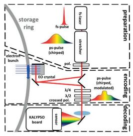
Figure 1: EOSD experimental setup at KARA.
