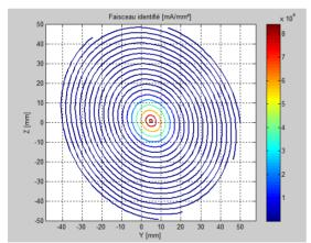
Figure 5: 2D profile of the beam for a current of 250 μA, focusing of 12 keV and 0 A in quadrupole.
