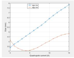
Figure 6: Influence of the quadrupole current on the beam
