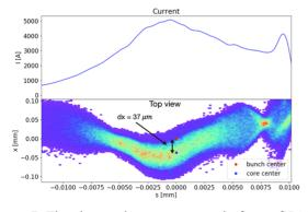
work may be used under the terms of the CC Figure 7: The electron beam parameter in from of SASE2 undulator, the beam energy 14 GeV, 250 pC [16].
