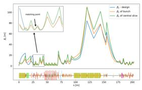
Figure 1:  $\beta_y$  of the first 200 m of the EuXFEL accelerator: design  $\beta_y$  (blue line),  $\beta_y$  of whole bunch from tracking with SC. (orange line),  $\beta_y$  of the central slice (green).
