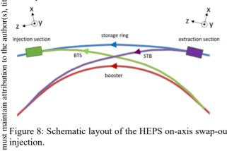
Figure 8: Schematic layout of the HEPS on-axis swap-out injection.
