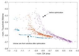
Figure 5: Optimization of the DA and Touschek lifetime, by varying only the multipole strengths.
