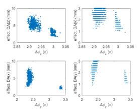
Figure 4: Phase advance between two focusing sextupoles in each 7BA of the found solutions without any constraints on the phase advance.
