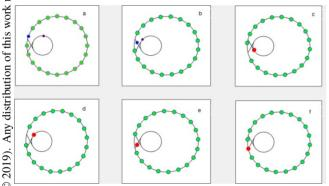
Figure 9: Process of replenishing a bunch in storage ring during HEPS operation.
