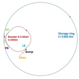
Figure 1: Schematic layout of the HEPS project.
