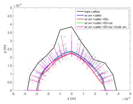
Figure 6: DAs of the HEPS storage ring, for the bare lattice, and for the case with practical errors. The colored curve represents the 20th-percentile smallest DA among the random error seeds.
