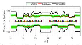
Figure 7: Local MAs of one super-period of the HEPS storage ring, for the case with the bare lattice and with practical errors.
