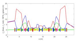
Figure 3: Optical functions and layout of one 7BA of the latest HEPS storage lattice.
