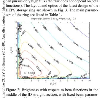
middle of the ID straight section, with fixed beam parameters, and with undulator parameters optimized at photon Content from this work may be used under the energy of 20 keV.
