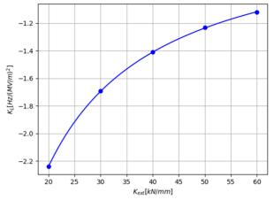
Figure 1: Lorentz force detuning (LFD) coefficient as a function of external cavity stiffness, cold cavity.
