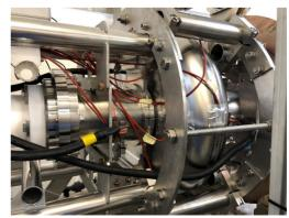
Figure 2: PIP-II FG001 single-cell during preliminary EP treatment at E. Zanon.
