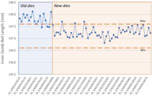
Figure 6: Example of scatter of measurements on length of Inner Dumb Bell before trimming. This is a typical plot available on the ESS Dashboard.
