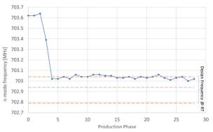
Figure 3: Frequency evolution during the cavity production cycle. The large variation at the beginning is due to the "bulk BCP" process.
