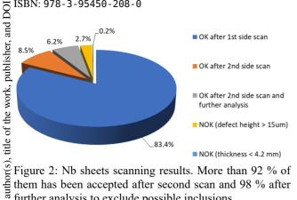
Figure 2: Nb sheets scanning results. More than 92 % of them has been accepted after second scan and 98 % after further analysis to exclude possible inclusions.
