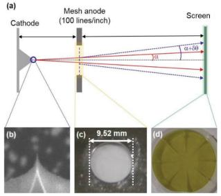
Figure 1: (a) A schematic of the experimental setup (b) The diamond nanotip, (c) the mesh anode, and (d) the AZO screen.
