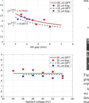
Figure 2: Measured and simulated divergence angles at different AK gaps and applied voltages. (a) The AK gap was varied from 3 to 6 mm, and the applied voltage was fixed at 40 kV. (b) For the 20 and 10 µm pyramids, the AK gap was fixed at 4 mm and 3.6 mm, respectively, while the applied voltage was varied.
