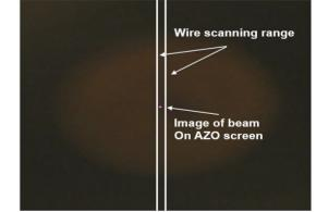
Figure 4: Snapshot of the beam at a distance of 16 mm from the magnetic center of the lens. The white bars indicate the wire scanning range.
