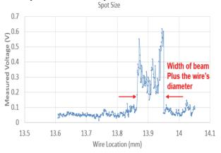
Figure 6: Graph of the measured voltage on the copper wire versus the location of the wire. Showing a spot size of  $5.72 \mu m$ .
