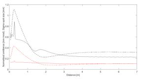
Figure 3: Beam envelope (dashed) and emittance evolution for 100 pC (black) at  $\sigma_r = 0.25$  mm and for 10pC (red) at  $\sigma_r = 0.13 \text{ mm.}$
