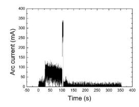
Figure 7: Arc current waveform under 1500V arc voltage.
