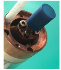
Figure 2: Installation of the cold cathode.
