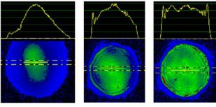
Figure 4: Laser transverse intensity distribution captured at the photocathode plane for a variable iris diameter of 1 mm and different transport beamline magnifications: M = 1.7 (left); M = 3.3 (middle); M = 5 (right). The top pictures show the projection of a horizontal section along the centre line.
