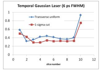
Figure 6: Slice emittance simulations when using laser pulses with a transverse uniform and truncated Gaussian
