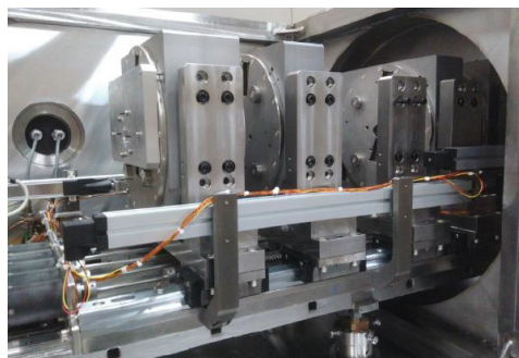
Figure 2: PMQs with their mechanical system.
